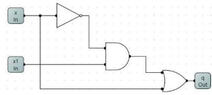
2). Implement the following truth table in Logic Circuit. Draw the circuit. Use sensor inputs and a probe for the output. What function does this circuit implement?
