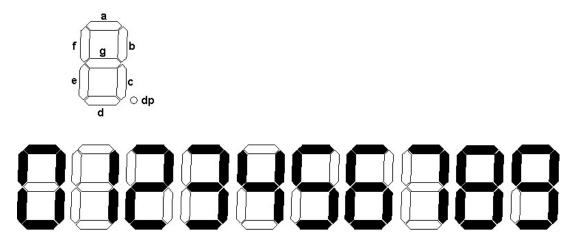
For example, the digit 4 has segments b,c,f and g lit. Internally, the device will receive a 4 bit binary code to represent these digits:
