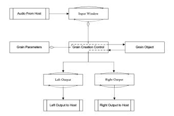
Figure 1: Granular Delay Engine
