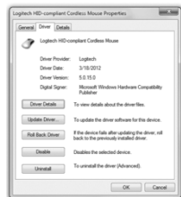
FIGURE 3-17 The Windows Device Manager offers access to device drivers. You can check if they are working and change settings. You can also check the device driver's version number and compare it with the most recent version posted online.
