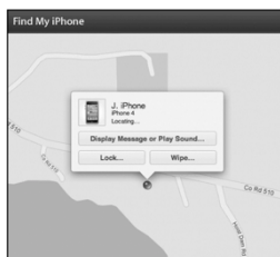
FIGURE 2-60 Find My iPhone can locate a missing phone and remotely lock it or delete its contents.
