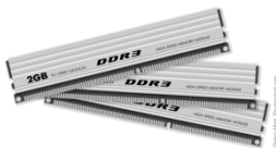
FIGURE 2-23 SDRAM is the most popular type of RAM in today's computers. It is typically available on a small circuit board. When adding memory to a computer, follow the manufacturer's instructions carefully.
