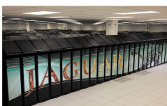
FIGURE 1-19 In 2010, a Cray XT5SHE computer named Jaguar was the fastest supercomputer. Using more than 18,000 processors, the Jaguar clocked peak performance speeds of 2.3 petaflops or 2.3 quadrillion operations per second.
